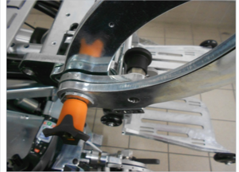
Fig. 29: Spring plunger latch unlocked
