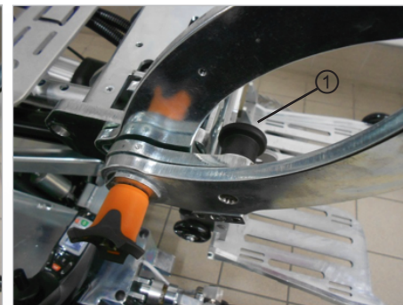
Fig. 32: Spring plunger latch locked
