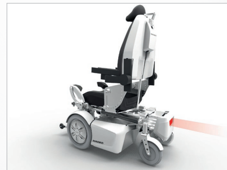
Fig. 10: Illumination at the rear
