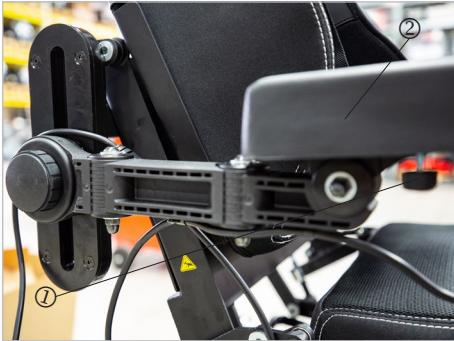
Fig. 17: Position of the armrest pad
