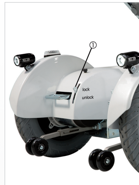
Fig. 38: Brake release lever (emergency release)
