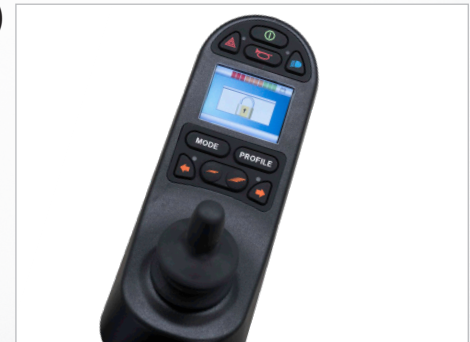
Fig. 109: Blocking the controls
