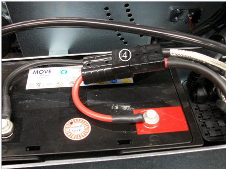
Fig. 56: Main Cable battery
