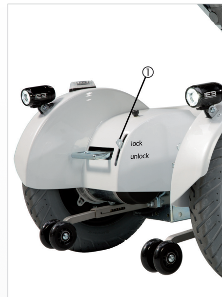
Fig. 42: Brake release lever (emergency release)
