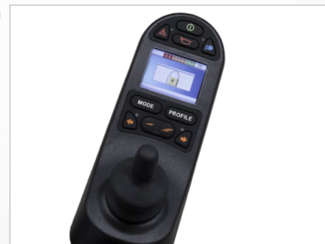
Fig. 101: Controls blocked – block symbol
