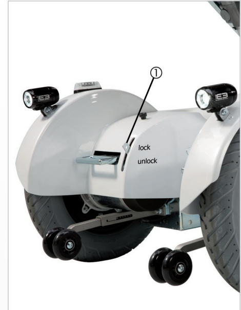
Fig. 29: Brake release lever (emergency release)
