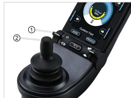
Fig. 78: Blocking the controls
