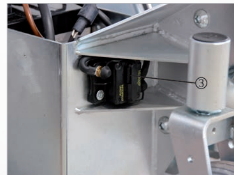
Fig. 111: Main safety switch
