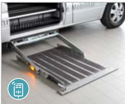
Digital, processor-controlled motion sequence – no mechanical limit switches!
