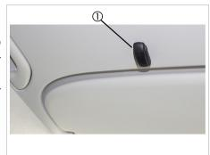
Abb. 50: Microphone, roof install.
