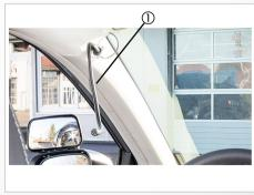
Abb. 51: Gooseneck microphone
