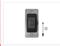
Abb. 33: Selecting driving gear
