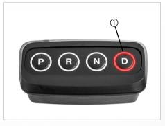
Abb. 30: Driving gear D
