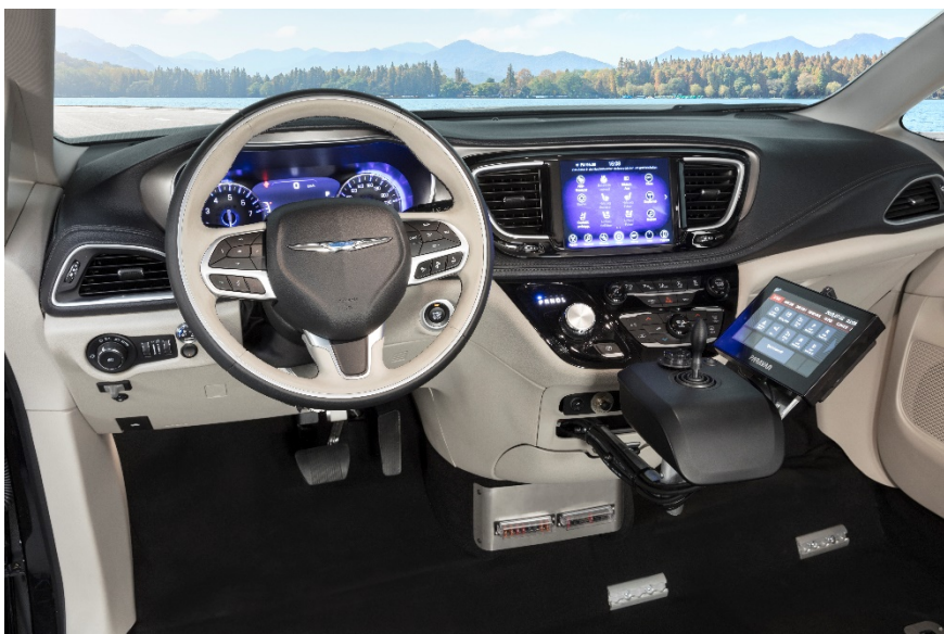
Chrysler Pacifica Space Drive Cockpit built by PARAVAN
