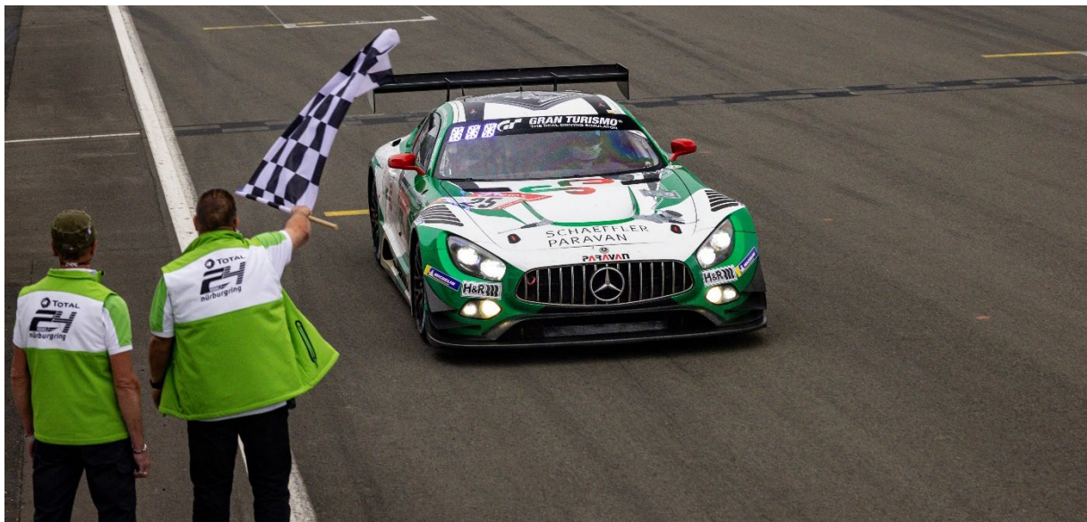
Historic finish: For the first time a GT3 car (Mercedes-AMG GT3) without a mechanical steering column successfully took part in the 24h Nürburgring. Photo GroupC photography
