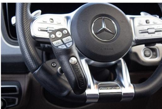
*The PARAVAN MultiMote can be adapted to completely different vehicle types. The freely programmable "A" button also allows functions such as cruise control or activation of voice control to be called up at the touch of a button. Photo: PARAVAN*
