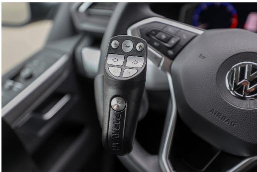
*The PARAVAN MultiMote can be used flexibly, whether on the steering wheel or on the handheld unit. This gives the user full control of the most important secondary functions without having to take his hand off the steering wheel. Photo: PARAVAN*
