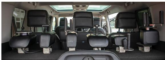
*The Space Drive driving and steering system offers many different solutions - whether 2-way joystick, 4-way joystick, mini steering wheel, or gas brake slider. The optimal attachment for gripping can also be adapted at the PARAVAN driving school. Photo: PARAVAN*
