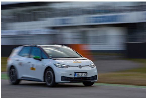
Thanks to Space Drive, the VW ID3 #18 does not require a mechanical connection between the steering unit and the steering gear. The 24h-e-competition is an ideal test field for testing the technology in a road vehicle. Photo: Schaeffler-Paravan
