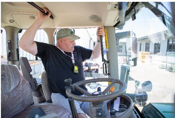
Handholds have been installed everywhere so that Edmund Ödamer can easily move into the passenger compartment at any time and has a secure hold everywhere. Photo PARAVAN
