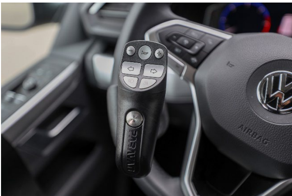
The PARAVAN MultiMote can be used flexibly, whether on the steering wheel or on the handheld unit. This gives the user full control of the most important secondary functions without taking his hand off the steering wheel. Photo: PARAVAN
