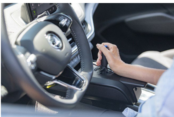
Svenja will control her vehicle with the Space Drive drive-by-wire system and two joysticks. With her left hand she operates the accelerator and brake, with her right she steers and can operate the most important secondary functions at the touch of a button. Photo: PARAVAN
