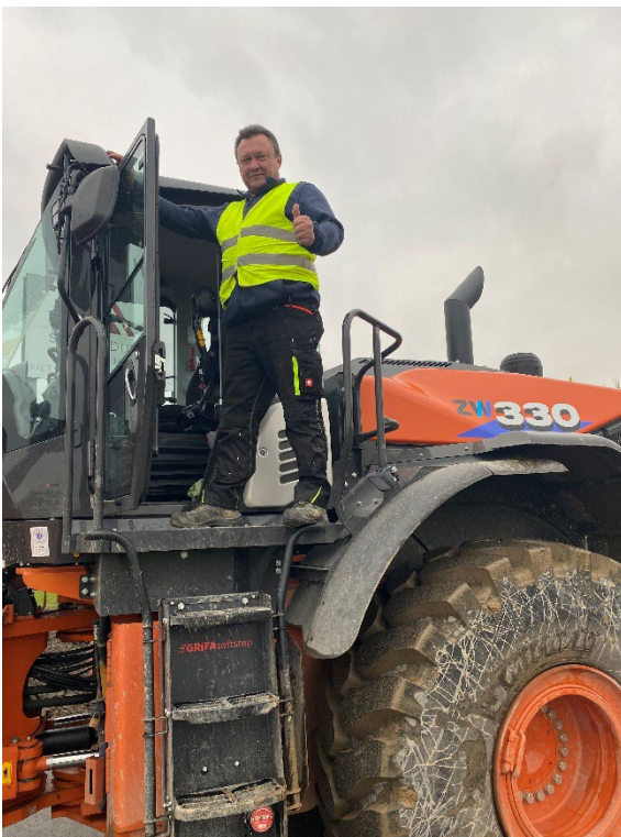
At last, Alexander Klems can go back to his usual job. Thanks to the drive-by-wire system, he can operate the throttle, which he also uses to move 4.8 cubic meters of construction materials in the bucket, with just two fingers. The Space Drive control unit and the actuators on the pedals do the rest for him. Photo: AG für Steinindustrie
