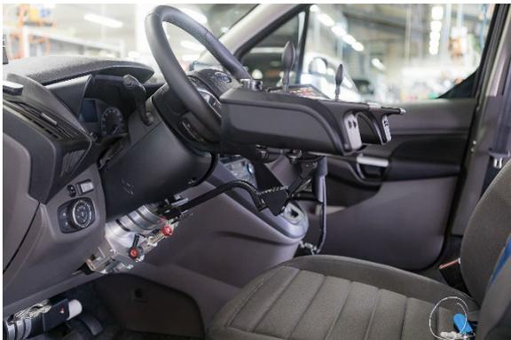
*The input devices are attached to the steering column via an anchor. If they are not needed, they can be removed at any time. Photo: PARAVAN*
