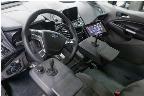
*Due to his disability, the joysticks for accelerator and brake as well as steering are very close together. This makes it difficult for other drivers who are not dependent on the individual input devices to reach the steering wheel. A mobile yet stable solution was needed. Photo: PARAVAN*
