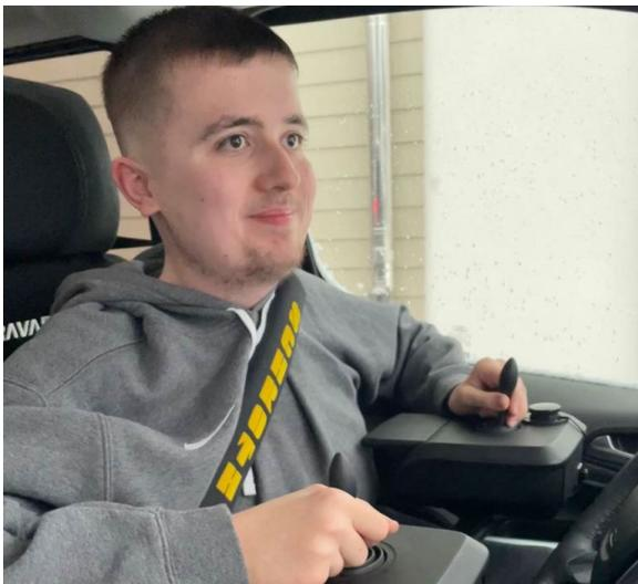
*Lukas is mobile again. His cockpit has a modular design. The joysticks that Lukas needs to drive can be removed at any time if someone else is sitting in front of the steering wheel. Photo: PARAVAN*
