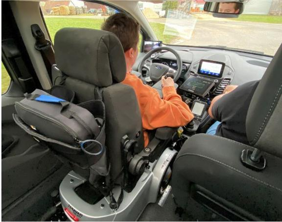
*Lukas drives his PARAVAN PR 50 over the ramp directly in front of the steering wheel, the wheelchair locks into the docking station and he's ready to go. Photo: PARAVAN*
