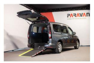
The VW Caddy Maxi 5 is equipped with a rear ramp and the corresponding attachments. This means that a wheelchair user can ride in the vehicle without any problems - whether active or power wheelchair, Photo: PARAVAN
