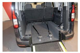
Also on board the barrier-free VW Caddy Maxi 5 for Avis is a complete wheelchair fastening system based on the power-knot principle as well as a three-point belt for the passenger in the wheelchair, Photo: PARAVAN
