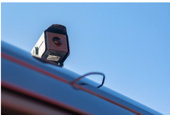
A high-resolution camera system positioned on the left side of the car provides a perfect all-round view of the left side of the vehicle and helps Katja achieve the mobility she had hoped for. Photo: PARAVAN
