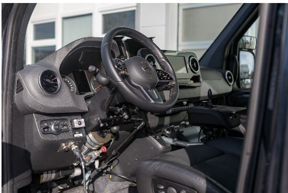
The new Mercedes Sprinter of the PARAVAN driving school offers many possibilities and can be converted very quickly, depending on requirements, from the simple mechanical slope control unit to the Space Drive electronic driving and steering system. Photo: PARAVAN
