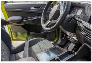
The goal of every PARAVAN mobility solution is flexibility and independence for the customer with a handicap. However, this also means that he or she must be able to get into the car without outside help. This is done here with the help of an electric door opening. The three-point belt is fitted in the door, so Ingrid Höhling can easily get into the car and drive off on her own. Photo: PARAVAN
