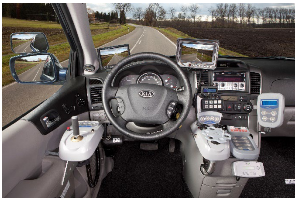
This is what the Space Drive cockpit of the first generation looked like. At that time, the secondary functions were still operated with many individual buttons. Photo: PARAVAN
