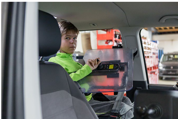
With the help of his own construction, he can move his table from the wheelchair, including the R-Net control, to the side. This leaves room for the 4-way joystick for the car. Photo: PARAVAN
