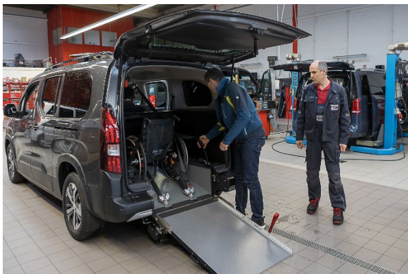
At the end, all the fastenings must be checked again properly, the switch for the electric good must be deactivated and the passenger must be correctly strapped in, photo: PARAVAN
