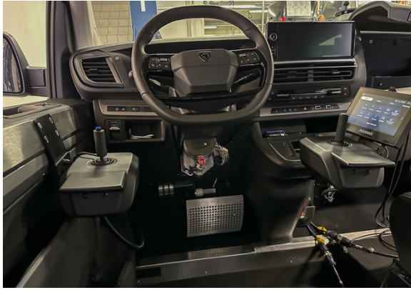
High-tech at the wheel: The Space Drive joystick control enables Benjamin to steer the vehicle precisely and safely – without a steering wheel or pedals. Photo: Paravan
