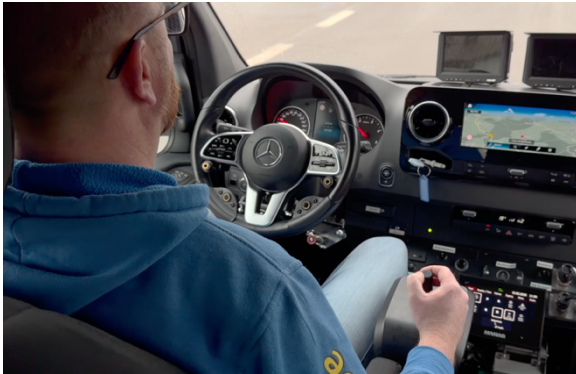
Driver training with Space Drive: Controlling the vehicle via joystick and digital driving functions in the training vehicle. Photo: Paravan
