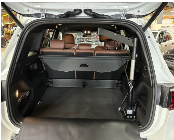
A look inside the trunk of the Mercedes GLB: Using a cable-operated loading aid, Serina can independently lift her wheelchair into and out of the vehicle. Photo: PARAVAN
