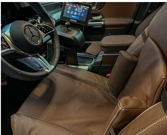
Customized driver's seat with joystick controls, the PARAVAN Touch System, and a custom-made backrest. Photo: PARAVAN
