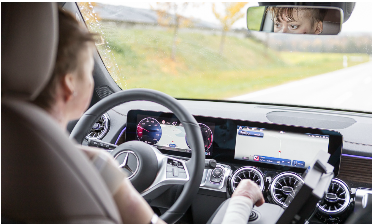
On the road in everyday life: Serina steers her Mercedes GLB using a 2-way joystick. The Space Drive electronic steering system enables her to drive independently and safely. Photo: PARAVAN
