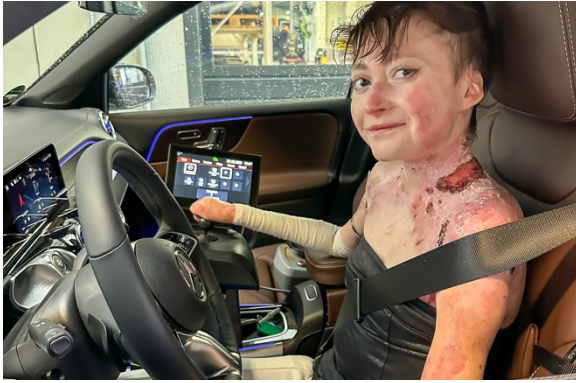
Serina controls her custom-modified Mercedes GLB with a 2-way joystick and Paravan's Space Drive electronic steering system. Photo: PARAVAN
