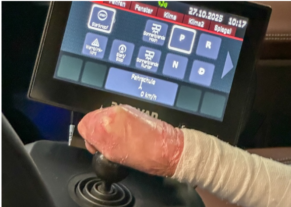
Serina controls her Mercedes GLB using a 2-way joystick. She operates vehicle functions such as the turn signals or sun visor via the PARAVAN Touch System or voice control. Photo: PARAVAN
