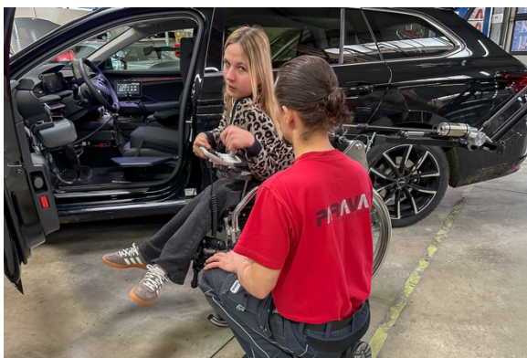
Adaptation of the wheelchair and the entry area for safe and independent transfer into the vehicle. Photo: Paravan.
