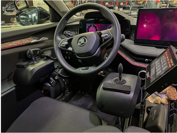
Custom vehicle adaptation in detail: Control via joysticks and Paravan Touch for maximum independence. Photo: Paravan
