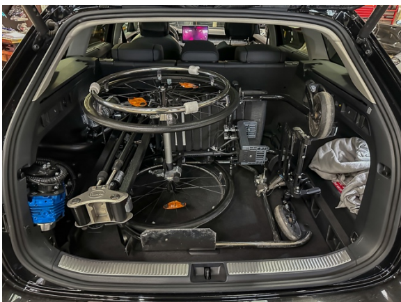
Automated wheelchair loading: The Robot 3000 enables safe stowage in the vehicle. Photo: Paravan
