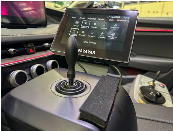
Intuitive operation: Paravan Touch and joystick enable control of all vehicle functions. Photo: Paravan
