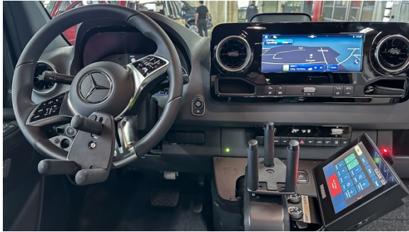
Customized controls in detail: A trident steering aid and gas-brake sliders enable precise control of the vehicle. Photo: Paravan
