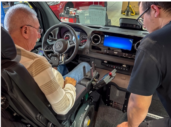
Individually tailored interaction: The wheelchair, vehicle, and controls are precisely adapted to the driver's needs. Photo: Paravan.
