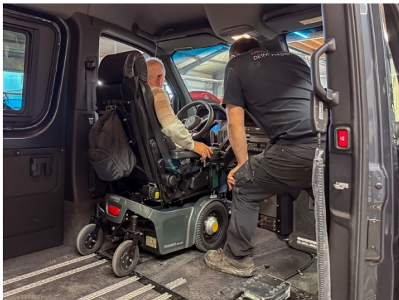
Seamlessly integrated: Cahit in the PR 50 electric wheelchair, which serves as the driver's seat in the vehicle. The wheelchair, vehicle, and controls are perfectly coordinated. Photo: Paravan
