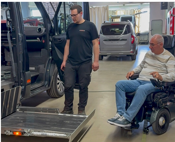
New solution for entry: Instead of the previous underfloor ramp, Cahit now uses a cassette lift to get into his vehicle independently. Photo: Paravan
