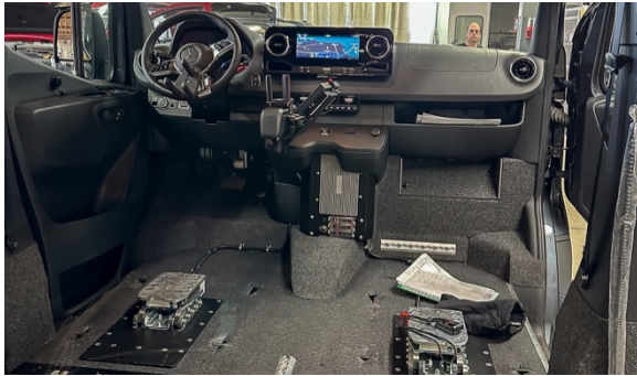
Flexible interior design: A rail system and docking stations allow the wheelchair to be securely integrated as the driver's seat. Photo: Paravan
