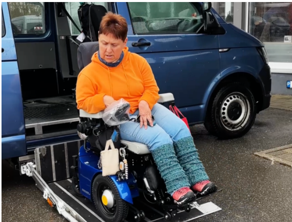
Seamless transition: With the cassette lift, Ulrike moves directly from her wheelchair into the vehicle—for maximum independence in everyday life. Photo: Paravan
