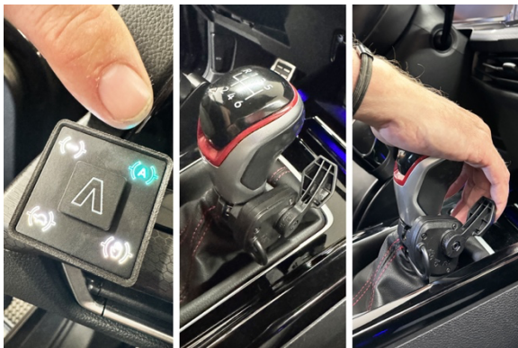
A new take on the manual transmission: The clutch function is electronically assisted, and various operating modes can be selected via a separate control panel. Photo: Paravan.
